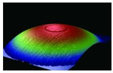
Figure 4. In the top image (a three-dimensional image of a UniCam Connector ferrule), fiber undercut has been precisely maintained to create a nearly smooth end-face. The factory-controlled polish leaves the surface nearly perfect. In the bottom image, this anaerobic connector ferrule end-face shows visible fiber protrusion and the hand polish has resulted in scratches over the entirety of the end-face.
