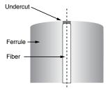
Figure 3. Fiber Undercut | Drawing ZA-1269
